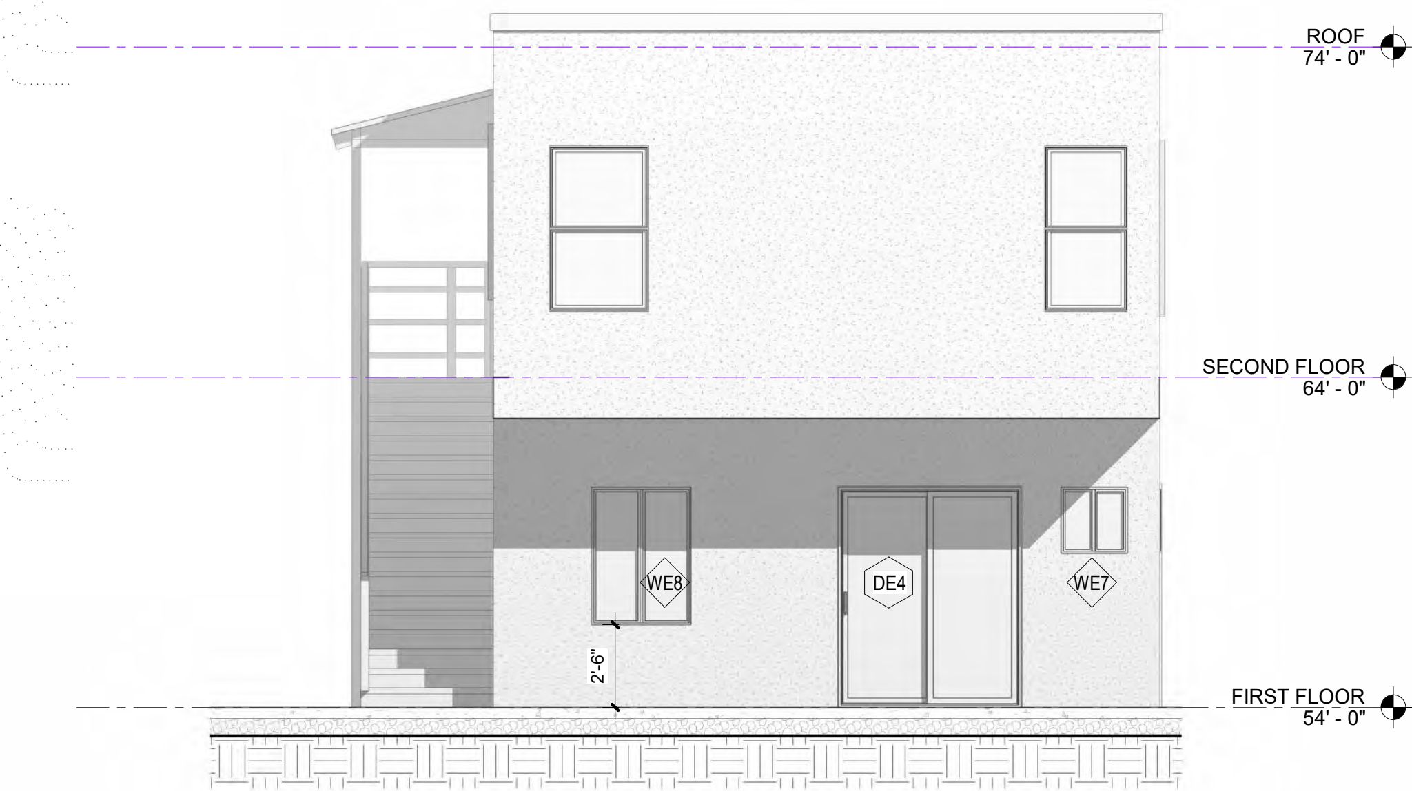
1 NORTH ELEVATION - ATTACHED ADU 1/4" = 1'-0"
